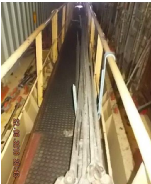
Figure 1(CB 280) Portable Stowage Hooks of the Kind that Failed
